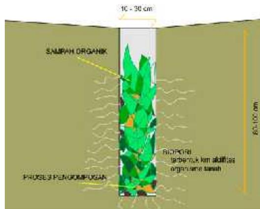
Gambar 1. Prinsip Lubang Resapan Biopori (LRB) hasil rekayasa manusia (Sumber: TBI, 2007).
